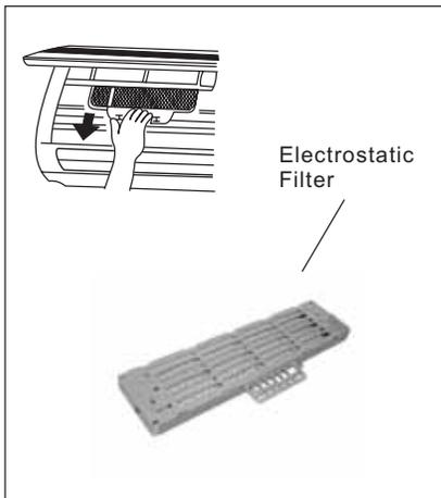
4. Remove the Electrostatic Filter from its support frame as shown in the Figure on the left (Not applicable to the units without electrostatic filter).
