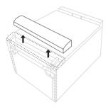
3 Remove the double-sided tape from the front strip.
